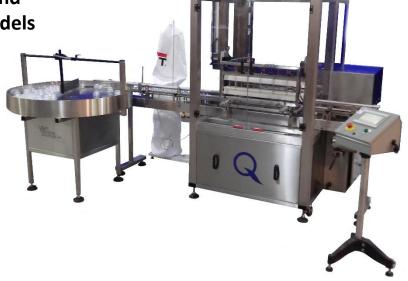
Bottle Vacuums use dual action nozzles to first blast the inside of each container with air to loosen dust and debris. Nozzles then seal the bottle opening and vacuum out debris to an easily cleanable waste reservoir. Bottle vacuums are available in both Automatic and Semi-Automatic models and are ideal for containers that are difficult to invert or otherwise rinse clean of debris.
